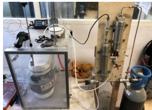
Figure 3.1 Production system for carbonated pastes
